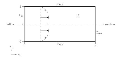
Figure 13.3: porousPoiseuille2d geometry with boundary patches and velocity profile.
