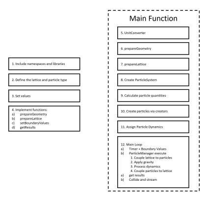
Figure 7.1: flow-chart of the example settlingCube3d
