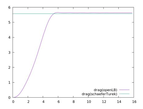
Figure 8.1: Gnuplot output of drag calculation in cylinder2d.
