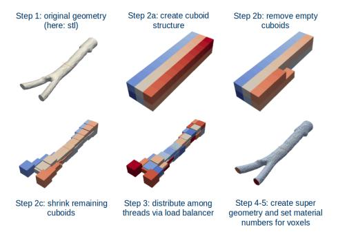
Figure 5.1: Six steps to create a Geometry. It starts by reading an stl file with the help of an STLreader and end with the creation of a SuperLattice.
