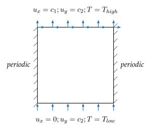
Figure 13.4: Schematic representation of the porous plate's simulation setup including it's boundary conditions
