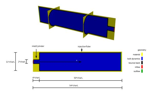
Figure 13.6: Cross section of a 3d geometry of nozzle3d in dependency of characteristic length charL.
