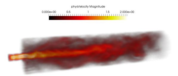
Figure 13.7: Physical velocity field after 200 seconds with preset parameters (Smagorinsky Model,  $C_S=0.15$ ,  $latticeL=\frac{1}{3}m$ ,  $Re_{inlet}=5000$ ).
