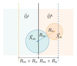
Figure 7.4: Overlap of the particle domains. Particles within a distance to of the sum of the two largest radii to a neighbour cuboid have to be transferred to this specific neighbour cuboid.
