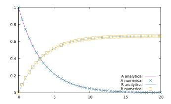
Figure 13.1: Solutions to concentration profiles in reactionFiniteDifferences2d.
