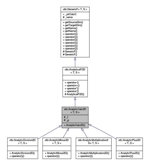
Figure 10.2: Inheritance for AnalyticCalc2D is shown.
