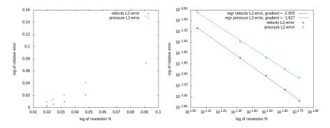
Figure 8.2: example of using regression to analyse polynomial errors (left: old, right: new implementation)
