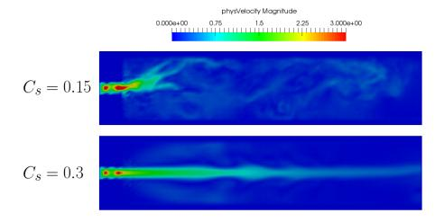
Figure 13.8: Increasing Smagorinsky Constant straightens turbulence.
