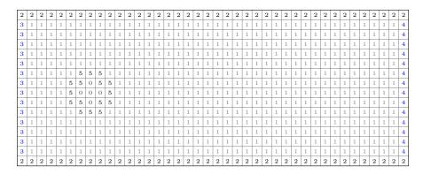
Figure 5.2: Lattice nodes of the geometry are associated to material numbers. Material number zero, one, two, three, for and five correspond to out of geometry, fluid, bounce back boundary, inflow, outflow and obstacle lattices, (1=fluid, 2=no-slip boundary, 3=velocity boundary, 4=constant pressure boundary, 5=curved boundary, 0=do nothing).
