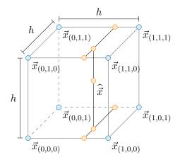
Figure 7.3: Trilinear interpolation.
